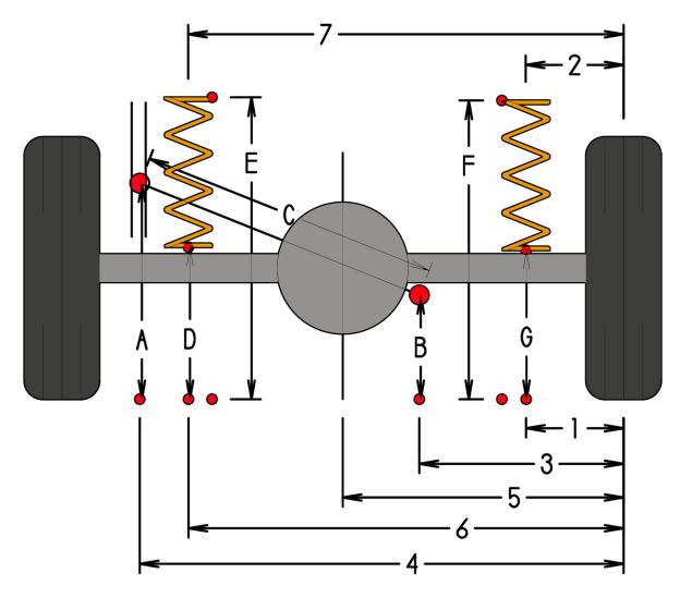
From the RR wheel side of the rotor, measure to each location marked 1,2-3. From the ground up measure the locations marked A,B-C.
